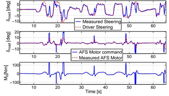
Fig. 10. From the top: a) driver turn wheel angle (dashed line) and real car turn wheel angle; b) AFS Motor command and its experimental measurement; c) Braking Moment command.
