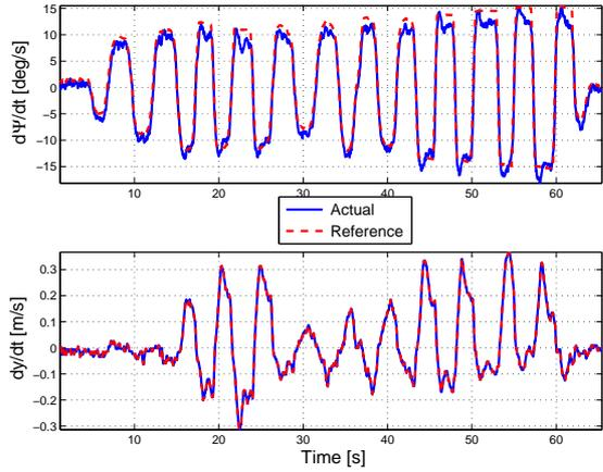
Fig. 4. Experiment 1: From the top: a) reference yaw rate (dashed line) and vehicle yaw rate (solid line); b) reference lateral speed (dashed line) and vehicle lateral speed [km/h] .
