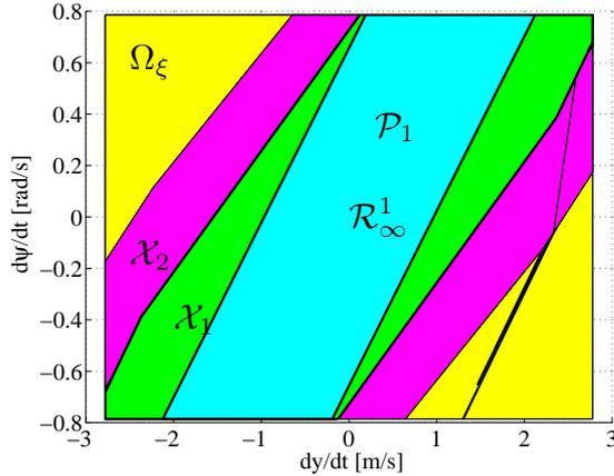
Fig. 2. Robust Control Invariant (RCI) set and 2-step controllable sets  $\mathcal{X}_k$  for  $\mu = 0.3$  and  $40 \leq v_x \leq 50$  [km/h].
