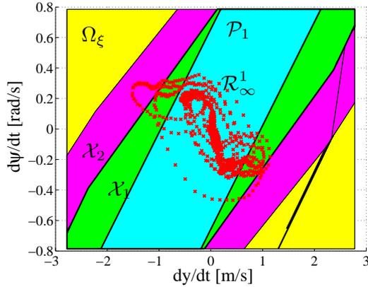
Fig. 9. State Trajectory depicted on  $\mathcal{R}_\infty^1$  and 2-step controllable sets  $\mathcal{X}_k$  for  $\mu = 0.3$  and  $40 \leq v_x \leq 50$  [km/h], and vehicle lateral speed [km/h] .
