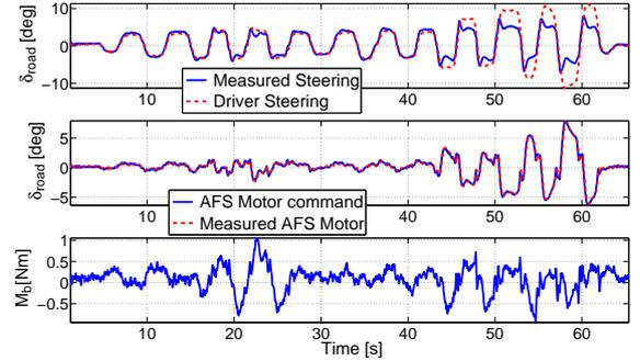
Fig. 6. From the top: a) driver turn wheel angle (dashed line) and real car turn wheel angle; b) AFS Motor command and its experimental measurement; c) Braking Moment command.
