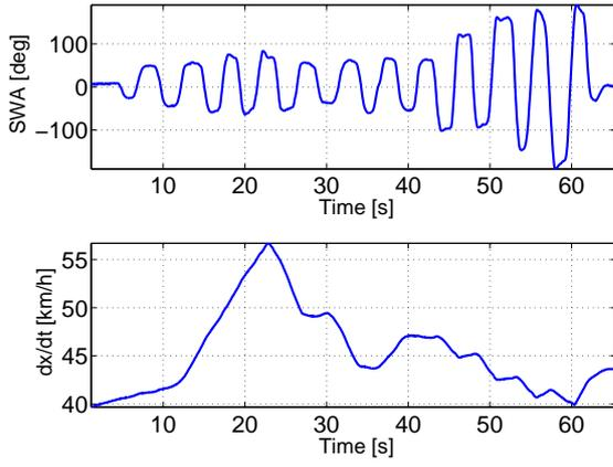
Fig. 3. From the top: driver turn wheel angle  $\delta_d$  in [deg] and vehicle longitudinal velocity in [km/h]
