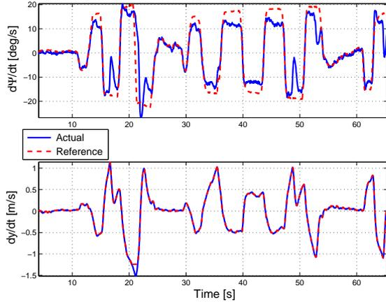
Fig. 8. From the top: a) reference yaw rate (dashed line) and vehicle yaw rate (solid line); b) reference lateral speed (dashed line) and vehicle lateral speed [km/h] .
