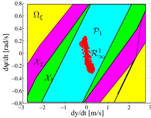
Fig. 5. State Trajectory depicted on  $\mathcal{R}_\infty^1$  and 2-step controllable sets  $\mathcal{X}_2$  for  $\mu = 0.3$  and  $40 \leq v_x \leq 50$  [km/h] and vehicle lateral speed [km/h].
